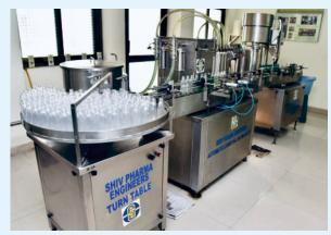
Liquid filling and cap sealing machine
