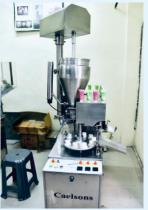
Semi-automatic tube filling, sealing & coding machine
