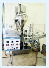
Automatic tube filling, sealing and coding machine
